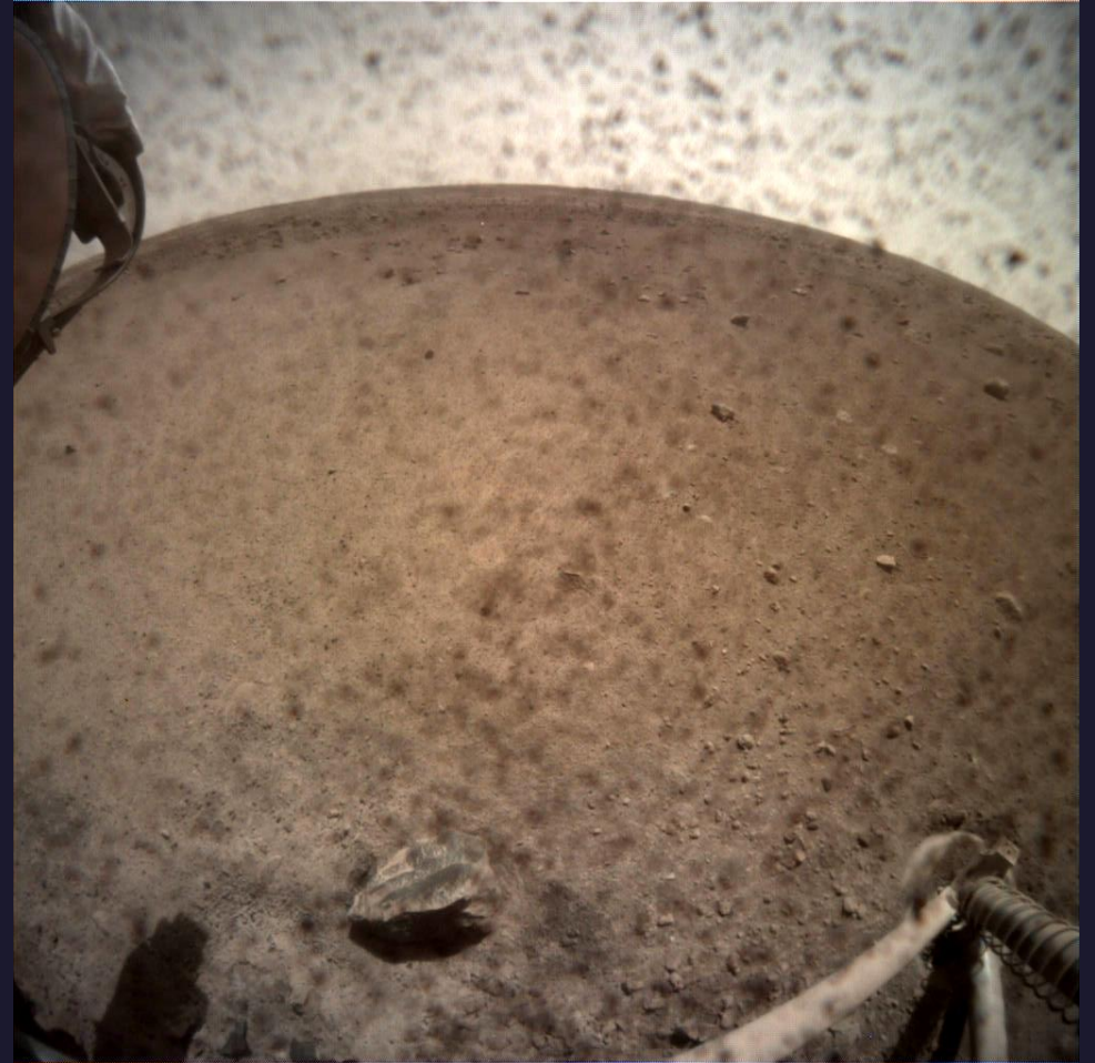
Mars Insight's Instrument Context Camera (ICC) before and after lens cover was opened (left and right images, respectively). The ICC was mounted below-deck, and the cover did not prevent all dust from getting on the lens.
